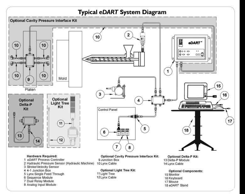
The eDART **flx** is for molders looking for an affordable system tailored specifically for automated abnormal part containment. In conjunction with the use of cavity pressure sensors, it can detect part abnormalities such as short shots, flash, sinks/voids, dimensional variations, warp and more, before the mold even opens. eDART **flx** provides a simple to use, fail-safe solution for sorting parts.
