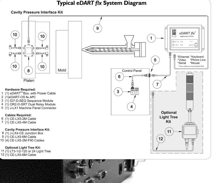
Lynx devices feed data to the eDART through digital communication, allowing for easy 'connect and go' usability. Job setup information only needs to be input the first time a sensor is connected, dramatically reducing setup times. The system recognizes the digital ID of the Lynx sensors and automatically calls up the job associated with that sensor. Lynx devices carry critical calibration information and self-checking diagnostics capabilities. Some of the common devices are listed below.
