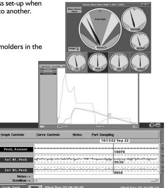
The eDART retains process and setup data for every mold run on a designated machine. Sensor configurations, process templates, alarm settings, and other setup information is automatically stored and can be easily shared with other eDARTs through a distributed network architecture. This unique ability to "share" information between eDARTs makes them interchangeable.
