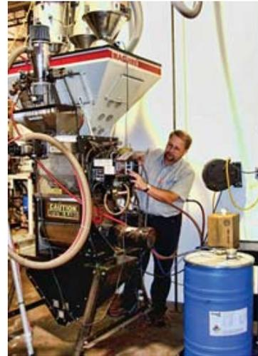
Manufacturing Manager Scott Pugh of Hayward adjusts control of Maguire Weigh Scale Blender. At lower right is Riverdale Color's Pump-in-a-Drum system, which meters liquid color into the blender.
